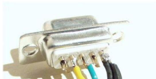
Figure 53 - Rear View of DB9
