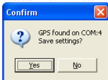
If the GPS is setup for 4800 baud (the standard value), then the TrackRanger PC must also be setup for 4800 baud.
